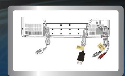
TIP: Create and attach labels to the cables, identifying the cables to make it easier to later connect the cables to the devices.
