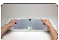
3. Pull up on the locking clip, then release it. Remove the base by gently sliding it away from the TV.
