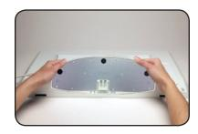
4. Move the TV with attached stand into an upright position and place on a flat, level, and stable surface.
