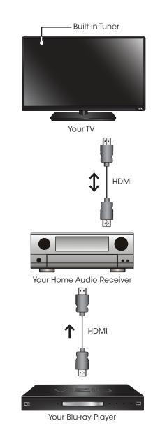
With an HDMI ARC setup, the audio connection between your TV and home audio receiver can be removed. The HDMI cable will transmit audio signals to and from your TV with an all-digital audio/video connection.
