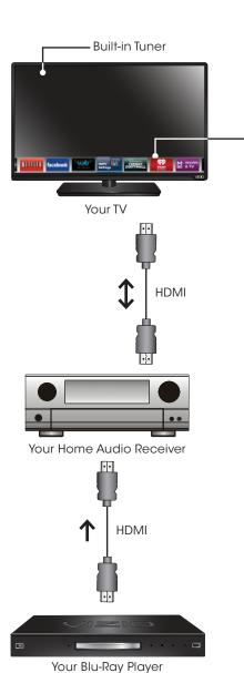
With an HDMI ARC setup, the audio connection between your TV and Home Audio Receiver can be removed. The HDMI cable will transmit audio signal to and from your TV with an all-digital audio/video connection.
