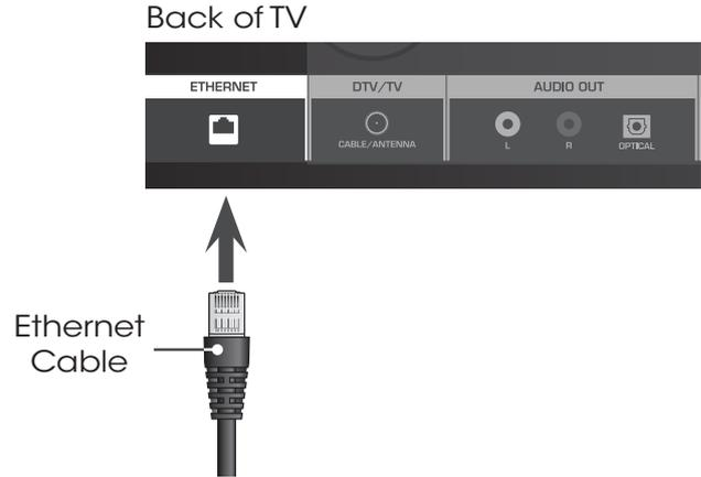
If you have a high-speed Internet connection, connect an Ethernet cable from your modem/router to the back of the TV as shown.
