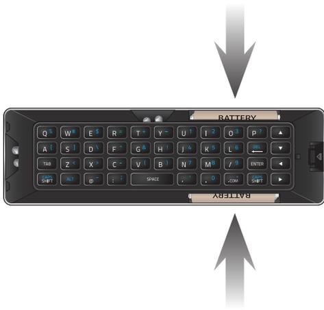
Insert two batteries into the remote control. Make sure that the (+) and (-) symbols on the batteries match the (+) and (-) symbols inside the battery compartment.
