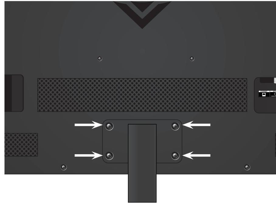
1. Align the neck piece with the bottom of the TV and slide it into place.
