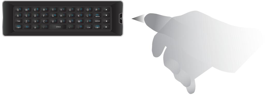
1. Press in on the button on the rear of the remote.
