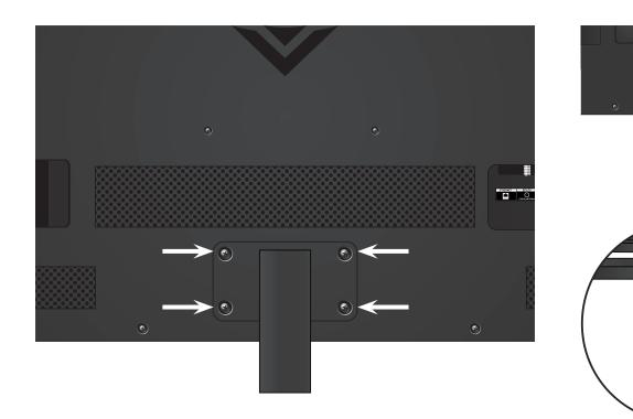
1. Align the neck piece with the bottom of the TV and slide it into place.
