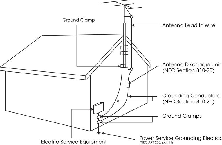
Power Service Grounding Electrode System (NEC ART 250, part H)
