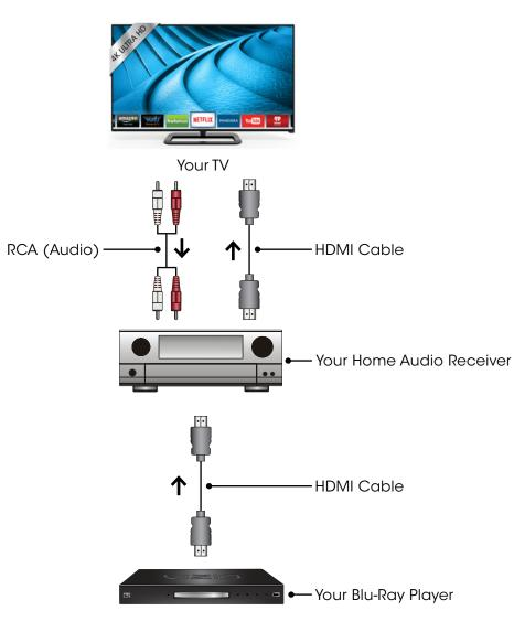
With an HDMI ARC setup, the audio connection between your TV and Home Audio Receiver can be removed. The HDMI cable will transmit audio signal to and from your TV with an all-digital audio/video connection.
