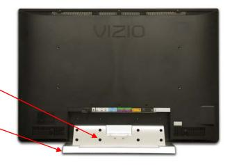
Now, the VU42L FHDTV10A can fit securely to a mount (sold separately) by utilizing the mounting holes in the center of the back panel of the TV. Please make sure to read the instructions of your specific mount to properly hang the VU42L FHDTV10A.
