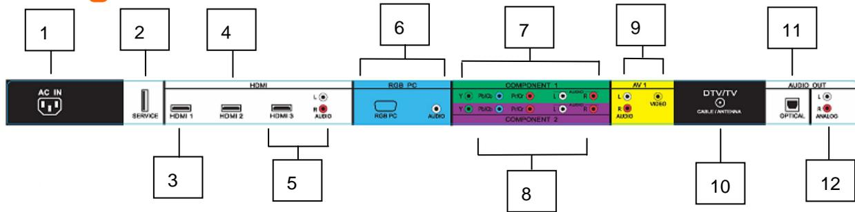
1. **AC IN** – Plug-in the supplied AC Power Cord here.
