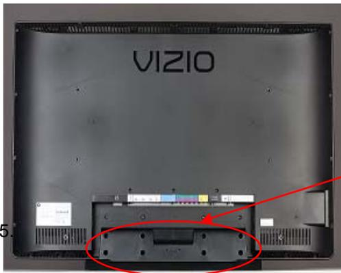
3. Remove the eight (8) screws so that the stand base can be removed.
