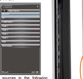
**Note:** When using the A/V input (usually, a composite signal) the video signal (yellow color coded cable) need to be connected to the green jack connector
