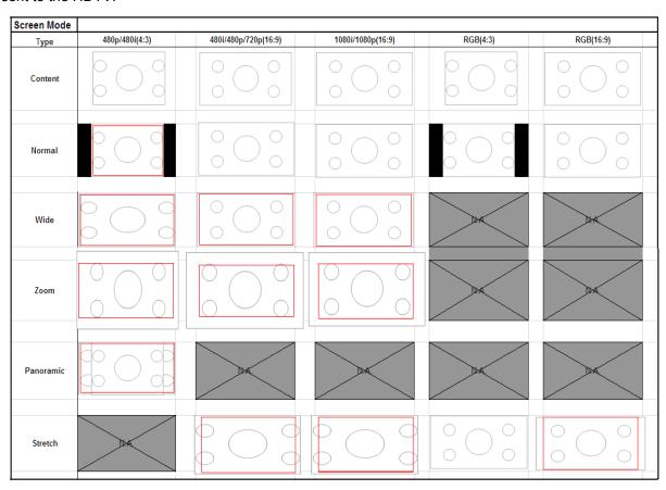
Note: The red lines show the video signal being overscanned.
