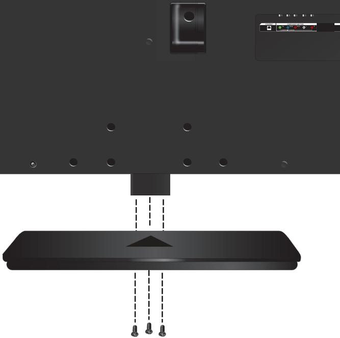
Align the base with the neck and tighten three (3) M6 12mm screws into the base with phillips screwdriver.
