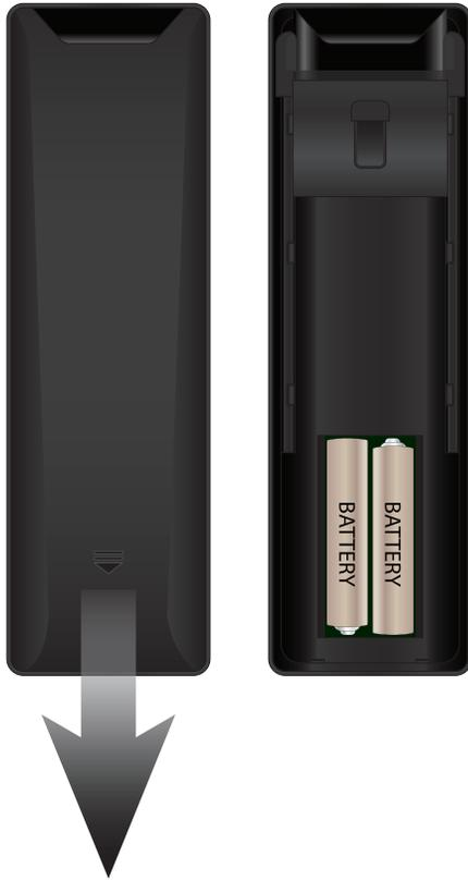
1. To remove the battery cover, press on the logo and slide the cover out.
