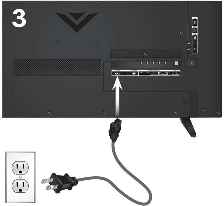
Connect the power cord to the back of the TV. The flat edge of the connector goes toward the side of the TV.
