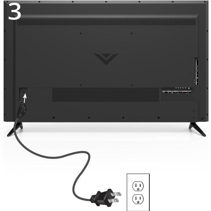
Connect the power cord to the back of the TV. The flat edge of the connector goes toward the outside of the TV.
