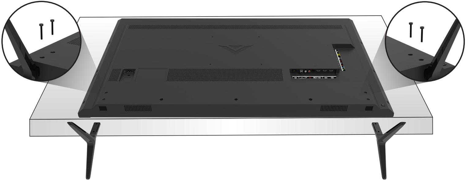
Insert the stands into the base of the TV. (The stands are identical.)
