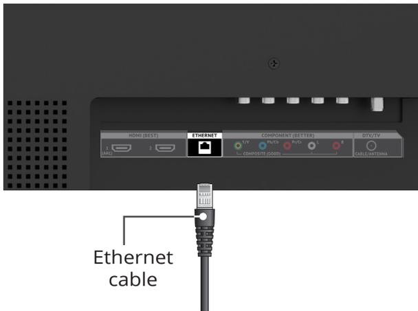
If you have a high-speed Internet connection, connect an Ethernet cable from your modem or router to the back of your TV as shown.
