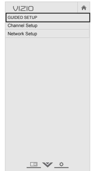
Press the **MENU** button to display the TV SETTINGS menu. Use the **Arrow** buttons to highlight **Guided Setup** and press **OK**. The GUIDED SETUP menu is displayed.
