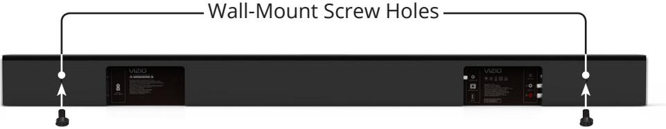
Insert the two wall-mount screws into the wall-mount screw holes, and then tighten them with a Phillips screwdriver.
