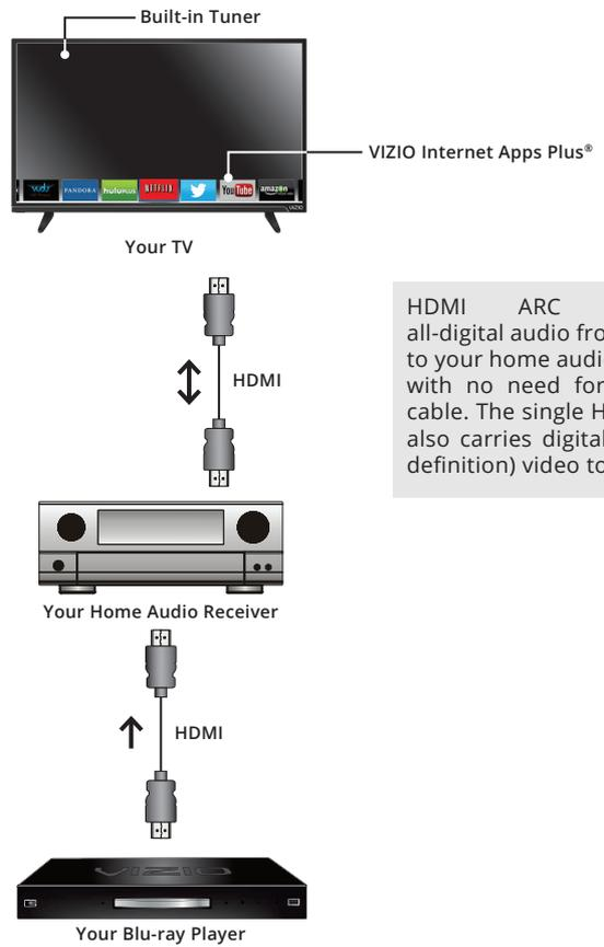
HDMI ARC transmits all-digital audio from your TV to your home audio receiver, with no need for an extra cable. The single HDMI cable also carries digital HD (high definition) video to your TV.
