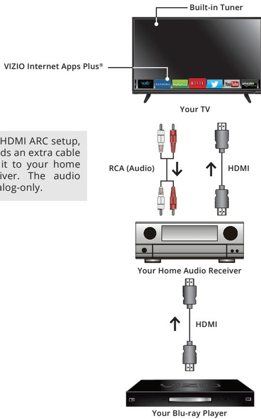
Without an HDMI ARC setup, your TV needs an extra cable to connect it to your home audio receiver. The audio signal is analog-only.
