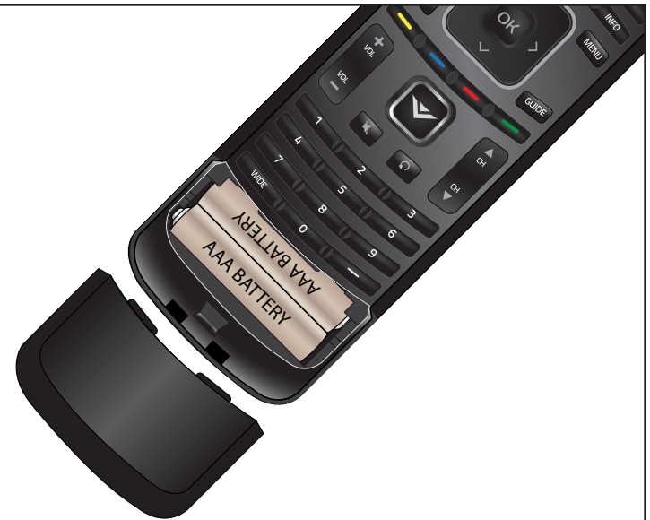
Replacing the Batteries
