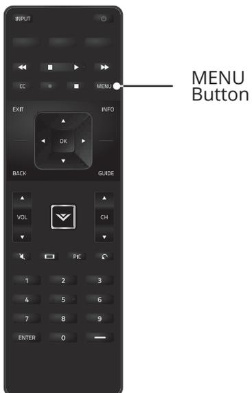
Press the **MENU** button on the Remote Control to display the TV SETTINGS menu.
