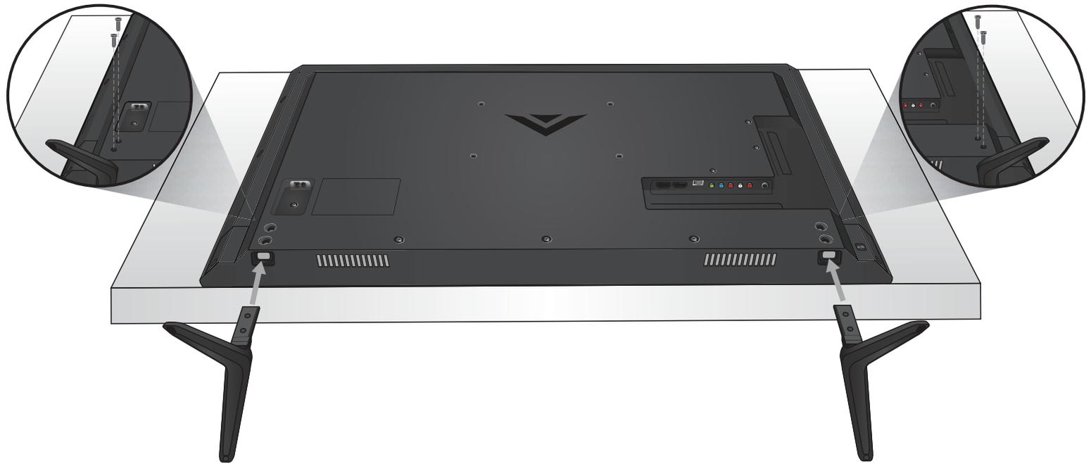
Insert the stands into the base of the TV. (The stands are identical.)
