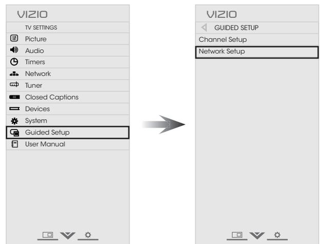
Press the **MENU** button to display the TV SETTINGS menu. Use the **Arrow** buttons to highlight **Guided Setup** and press **OK**. The GUIDED SETUP menu is displayed.
